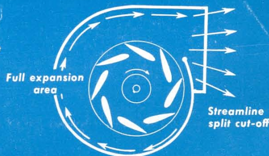
Proportioned to take full advantage of airfoil wheel
