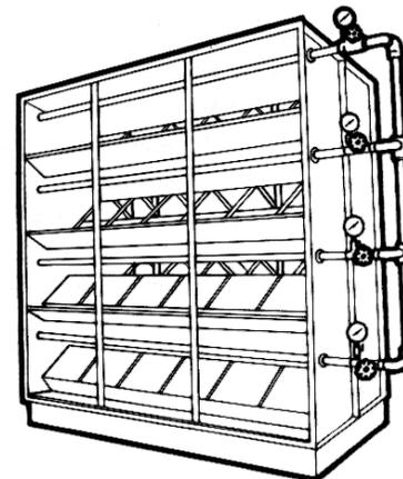
Illustration shows a cell type cell standard unit incorporating special elements in a 20”\*20”\*8” deep casing . Illustration (right) shows a standard cell type air washer with cell type cells removed from two of the banks.
